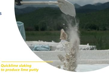
types of building lime that are used in the building sector are **certified according to EN459.** This describes all the different types of commercially available products and their specifications for quality control and proper application. Some of the environmental benefits of the use of lime, especially the air-hardening type, are the following:
